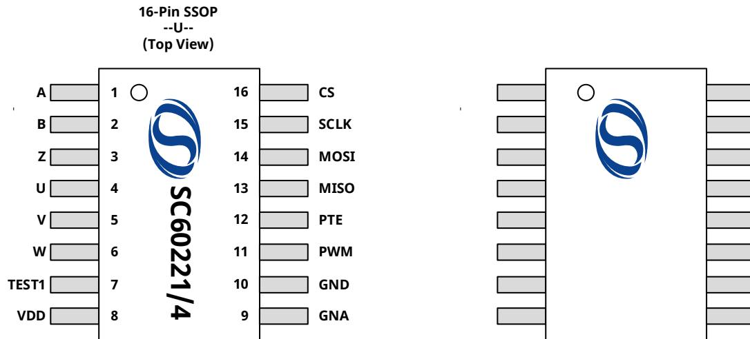
Fig2: SC60221/4 Terminal Configuration
