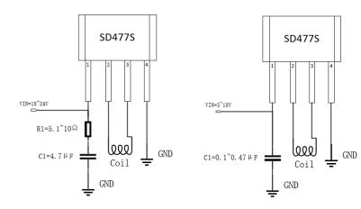
Note 3: When the power pulse is relatively large, Must use least C1=4.7 $\mu$ F(ceramic capacitor) capacitor & R1=5.1~10 $\Omega$  for the decoupling between VIN and GND and place the capacitor as close to the IC as Possible. C1 is an optional capacitor, which can enhance the reliability during hot swap.
